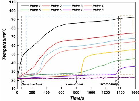
Fig 3 Temperature changes of the PCM at point 1-8 during the whole phase change process
