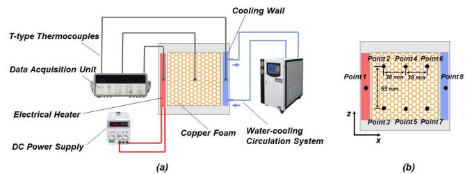
Fig 2 (a) Experimental test apparatus, (b) Coordinates of 8 T-type thermocouples
