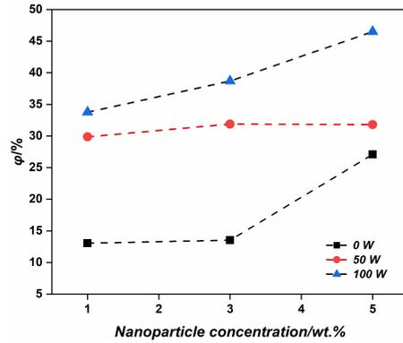
Fig 4 Reduction index ( $\varphi$ ) of melting time of nano-PCM under the effect of ultrasonic power and  $\text{TiO}_2$  nanoparticle
