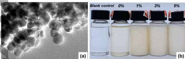
Fig 1 (a) TEM image of  $\text{TiO}_2$  nanoparticles, (b) Nano-PCM suspension with different nanoparticle concentrations
