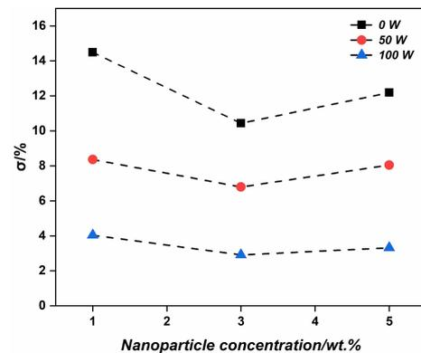
Fig 5 Temperature reduction index ( $\sigma$ ) of  $T_e$  of nano-PCM under the effect of ultrasonic power and  $\text{TiO}_2$  nanoparticle
