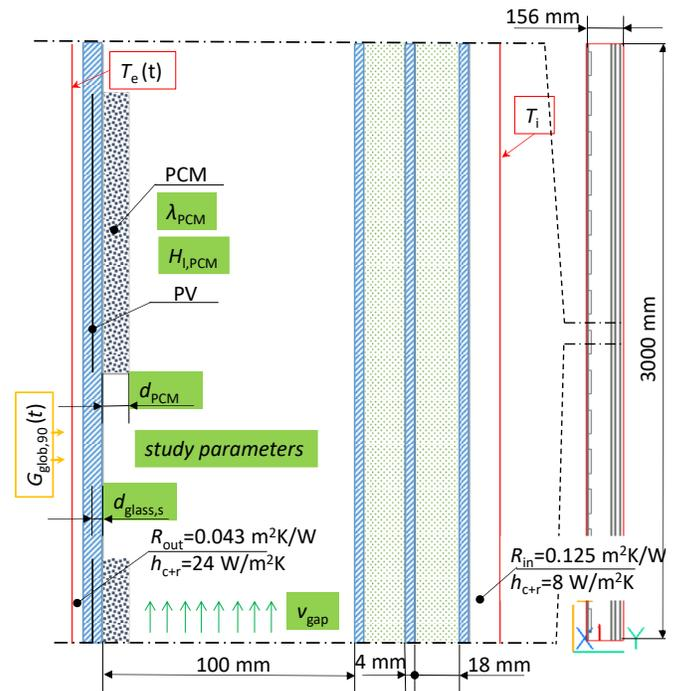
Fig 1 CFD model scheme with boundary conditions, varying parameters are presented in green frames.
