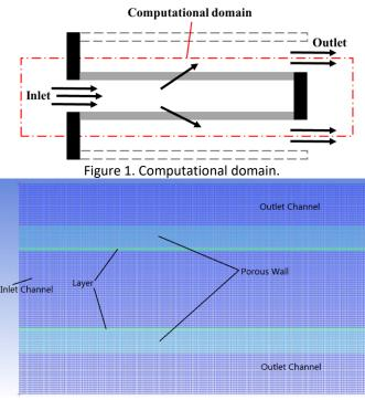
Figure 2. Grid diagram of DPF close to inlet.
