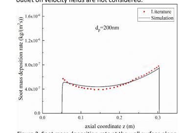
Figure 3. Soot mass deposition rate at the wall surface along the axial coordinate.
