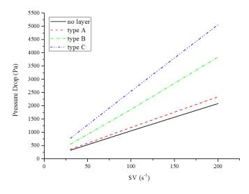
Figure 5. Pressure drops of homogeneous and heterogeneous wall structure DPFs.
