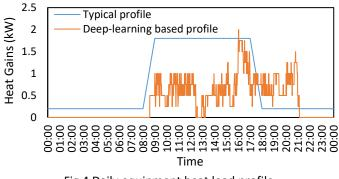
Fig 4 Daily equipment heat load profile
