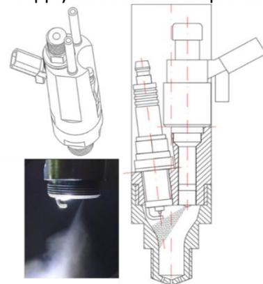
Fig. 2 Structure of the pre-chamber
