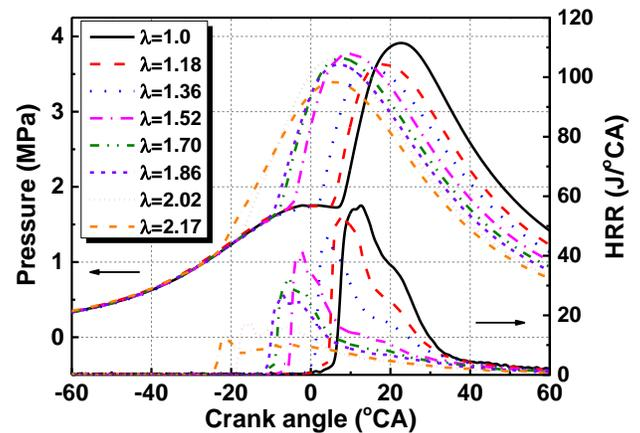
Fig. 6 In-cylinder pressures and HRRs of TJI with various excessive air coefficient
