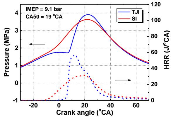
Fig. 5 Combustion comparison between TJI and SI at excessive air coefficient of 1.0
