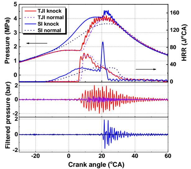
Fig. 8 In-cylinder pressures, HRRs and pressure oscillations of TJI and SI combustion modes
