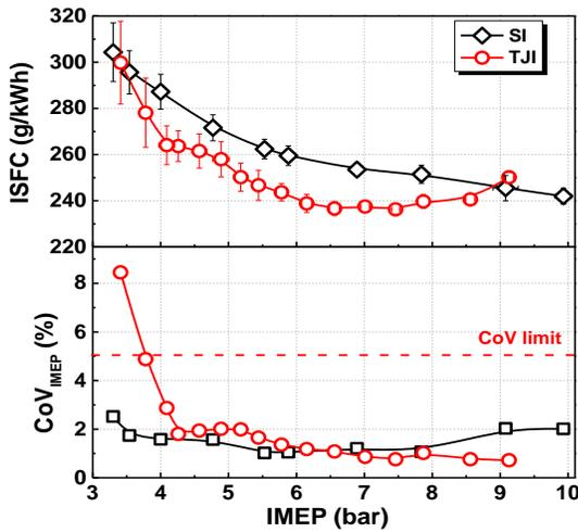
Fig. 4 Comparison between SI and TJI on ISFC and  $CoV_{IMEP}$
