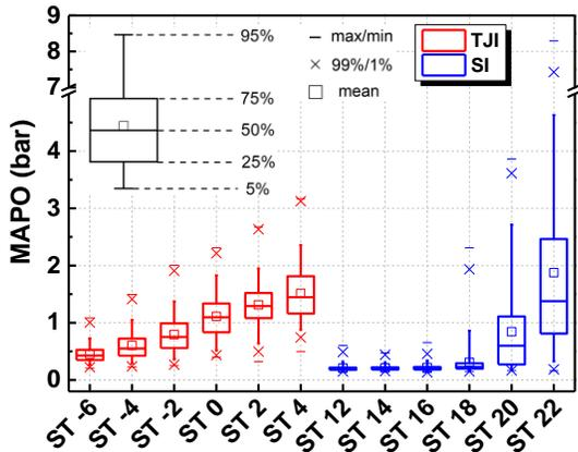
Fig. 7 MAPO distributions of TJI and SI combustion modes against spark timings
