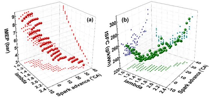
Fig. 3 IMEP and ISFC of TJI combustion with different spark timings and lambdas
