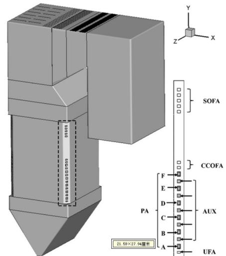
Fig 1 Schematic of the boiler and burner arrangement
