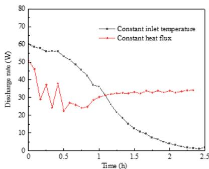
Figure 5. Discharge rate resulting from two discharging methods.
