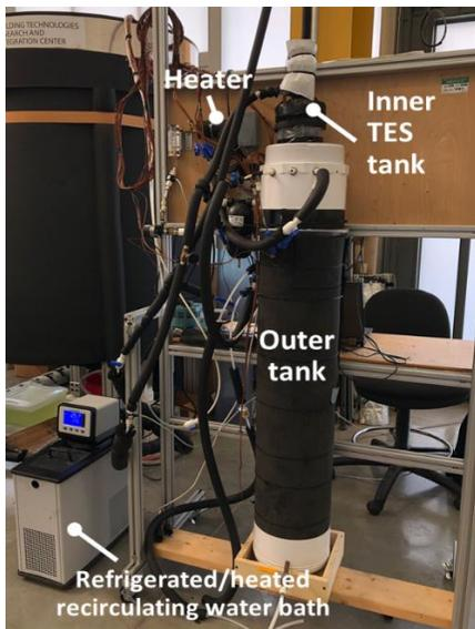
Figure 2. Photo of the experimental apparatus for characterizing performance of a lab-scale DPUTB.
