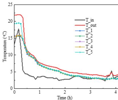
Figure 3. Inner tank temperature during the charging test.
