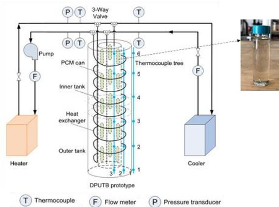
Figure 1. Schematic of an experimental apparatus for characterizing performance of a lab-scale DPUTB.
