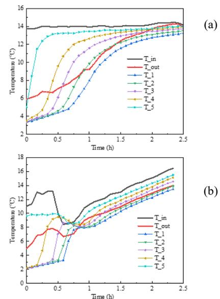
Figure 4. Inner tank temperature during discharging tests in different discharging methods: (a) with a constant inlet water temperature; and (b) with a constant heat flux.
