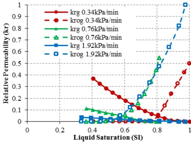
Fig. 4. Relative permeability curves of case 1 to case 3
