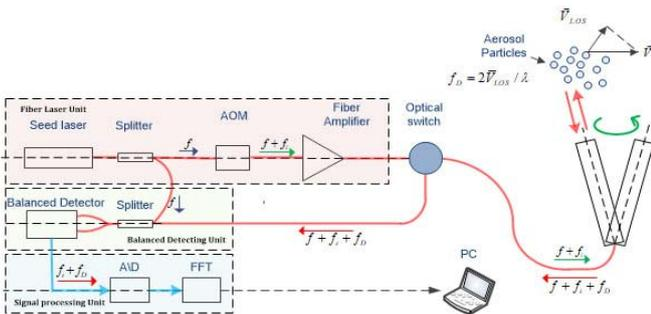
Fig. 2. Wind Lidar System Schematic
