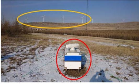
Fig. 4. Wind3D 6000 and the target wind turbines (Wind3D 6000 is circled by red line; WT10-1, WT10-2, WT10-3 and WT10-4 are the target turbines and are circled by the yellow line)
