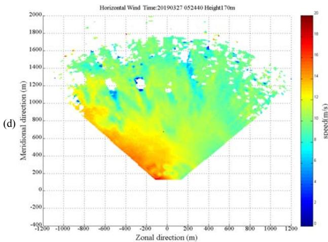
Fig. 5. Measurements of wake effect at a series of heights: (a) at the height of 65 m; (b) at the height of 100 m; (c) at the height of 135 m and (d) at the height of 170 m.
