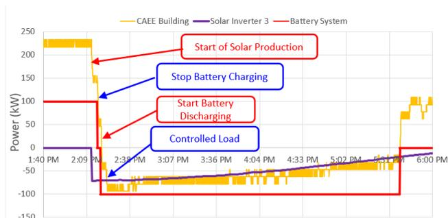
Fig. 7. CAEE Building demand deduction and net power fed back to the grid on RPU's voluntary load shedding request
