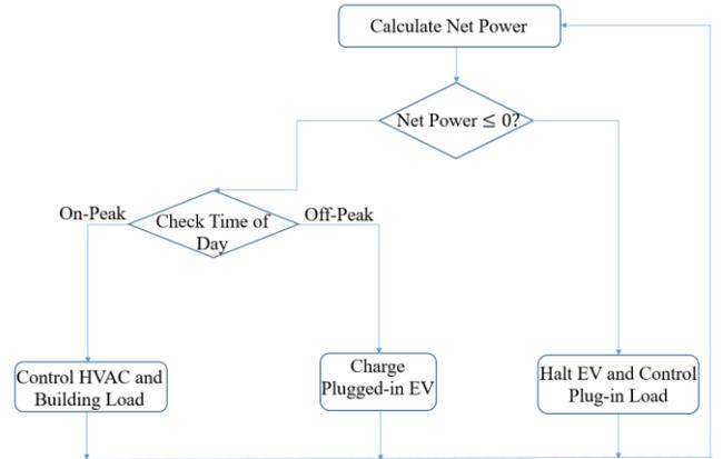
Fig. 3. Admin Microgrid Proposed Strategy: While Trolley is unavailable
