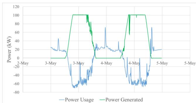
Fig. 5. The net zero administration building: PV generation and usage
