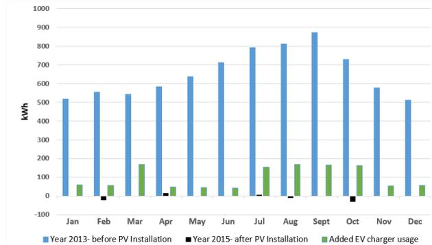
Fig. 6. Net zero demonstration: CE-CERT Administration Building daily average electricity usage from grid before and after PV installation
