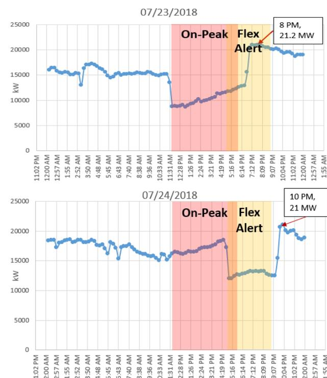
Fig. 8. UCR campus load before and after Flex alert actions
