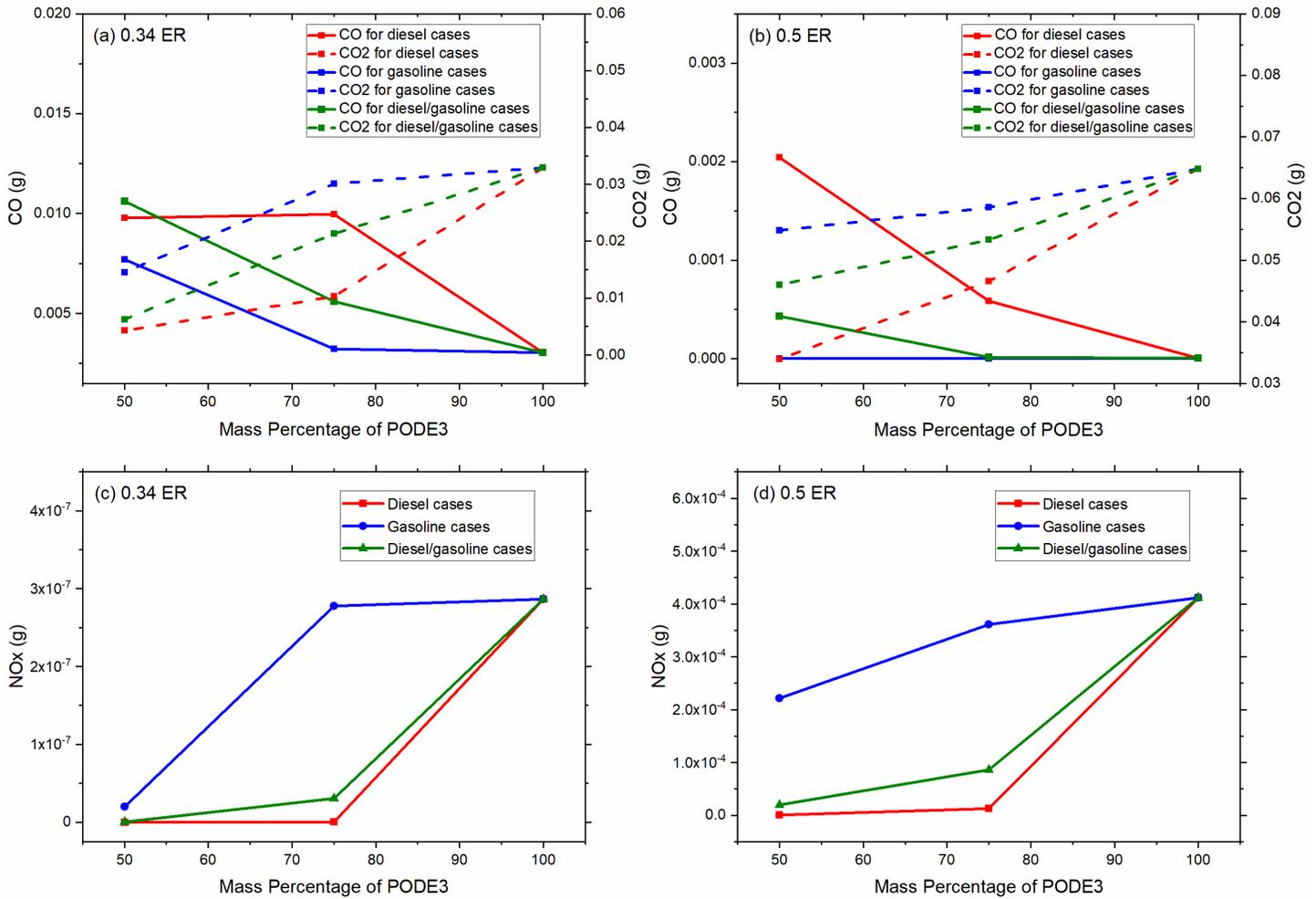
Figure 4 Emissions against mass percentage of PODE<sub>3</sub> of (a) CO and CO<sub>2</sub> at 0.34 ER, (b) CO and CO<sub>2</sub> at 0.5 ER, (c) NOx at 0.34 ER and (d) NOx at 0.5 ER.
