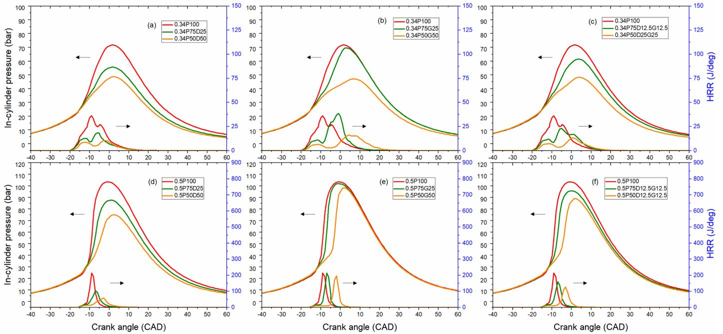
Figure 1 In-cylinder pressures and HRRs for (a) PODE<sub>3</sub>/diesel blends at 0.34 ER, (b) PODE<sub>3</sub>/gasoline blends at 0.34 ER, (c) PODE<sub>3</sub>/diesel/gasoline blends at 0.34 ER, (d) PODE<sub>3</sub>/diesel blends at 0.5 ER, (e) PODE<sub>3</sub>/gasoline blends at 0.5 ER and (f) PODE<sub>3</sub>/diesel/gasoline blends at 0.5 ER.
