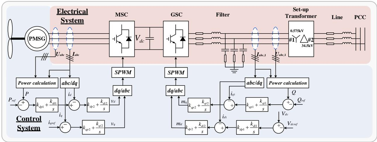
Fig 1 Configuration of the PMSG wind turbine
