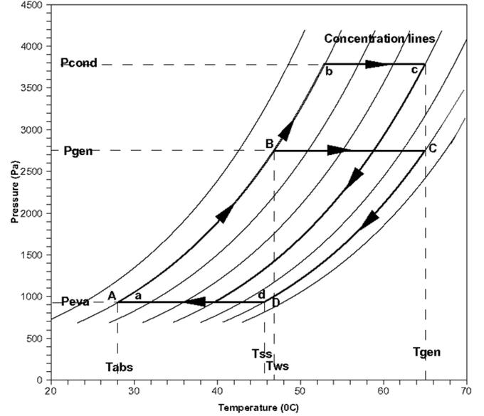
Fig 2 Solution concentration difference between the absorber and generator in an absorption cycle (abcd) and an integrated AD-AB cycle (ABCD) in P-T-X diagram.
