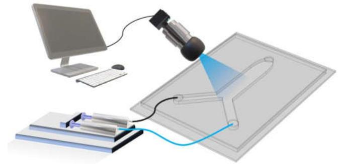
**Figure 1** Experimental setup for ion diffusion measurements.
