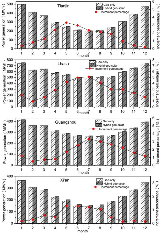
Fig. 3. Stand-alone geothermal plant and hybrid power plant time-by-time simulation calculation results, Scenario 1.
