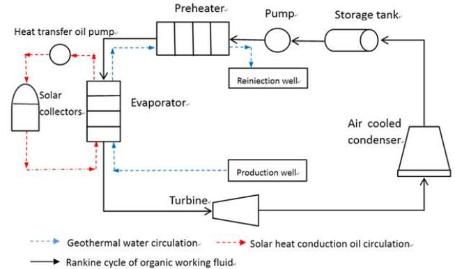
Fig. 1. Schematic diagram of the hybrid solar-geothermal power generation system
