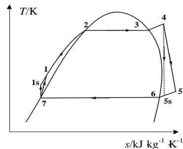
Fig. 2. T-S diagram of an ORC system
