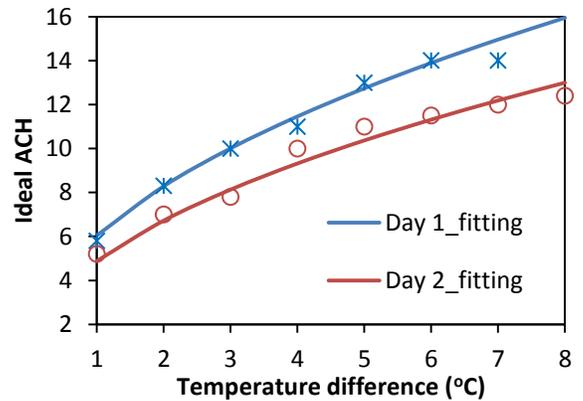
Fig 5 Fitting results of ACH on simulated days
