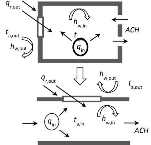
Fig 1 Heat transfer processes in two-plate room model
