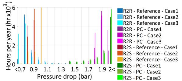
Fig 2 Pressure gradient at a consumer substation
