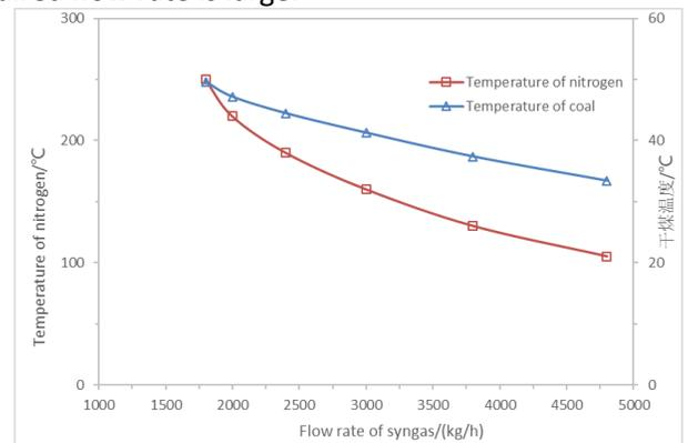
Fig 3 Relationship between circulating gas temperature and minimum flow rate and dry coal outlet temperature
