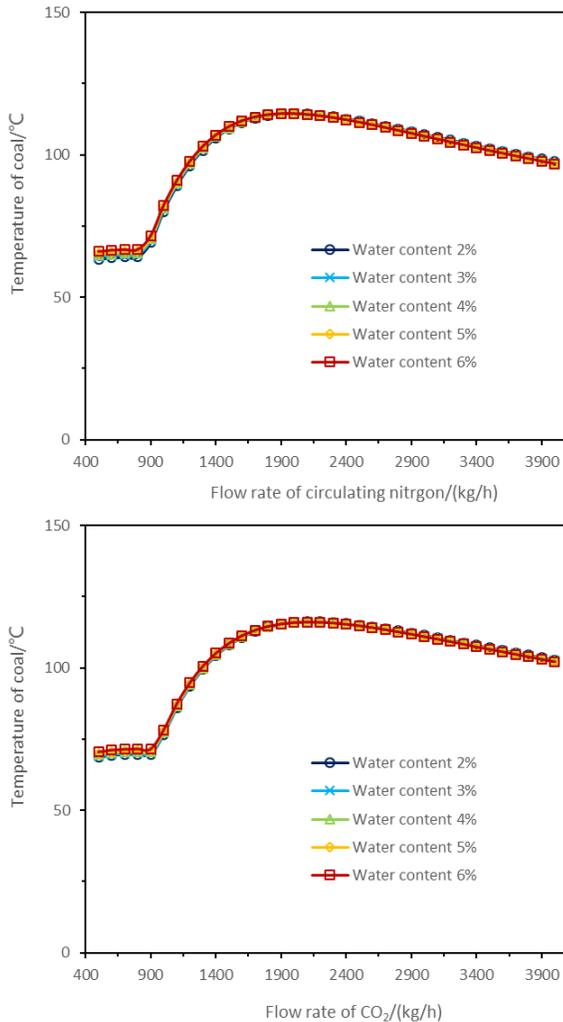
Fig 4 Effect of circulating gas water content on dry coal outlet temperature
