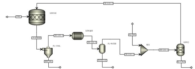
Fig 1 Dry quenching coke waste heat recovery model process
