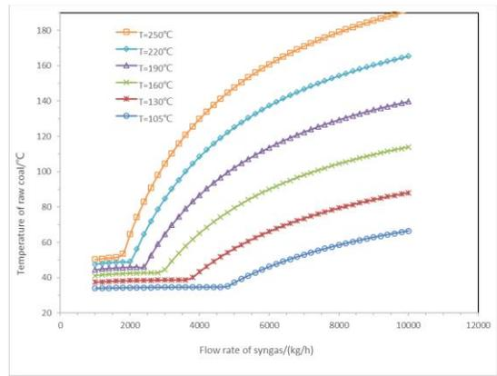
Fig 2 Effect of cycle gas temperature and flow rate on dry coal outlet temperature
