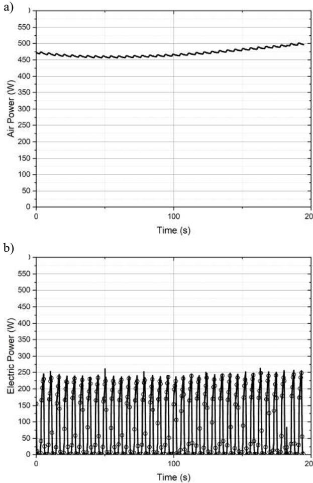
Fig 2 Experimental data: a) Air power; b) Generated electric power.
