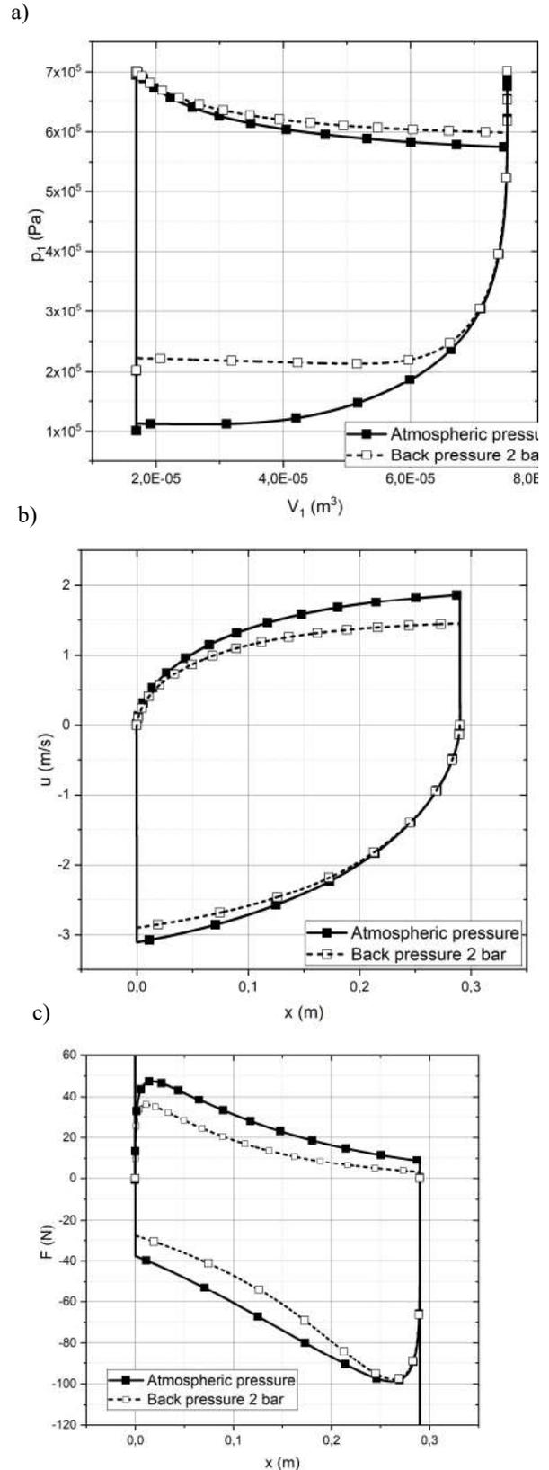
Fig 3 Computational results for pneumatic cylinder: a) Pressure-volume mapping; b) Velocity-displacement mapping; c) Force-displacement mapping.
