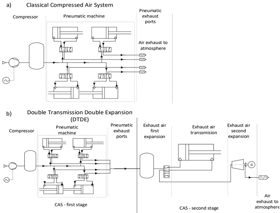
Fig 1 Topology of Compressed Air System: a) Classical; b) Double Transmission Double Expansion.
