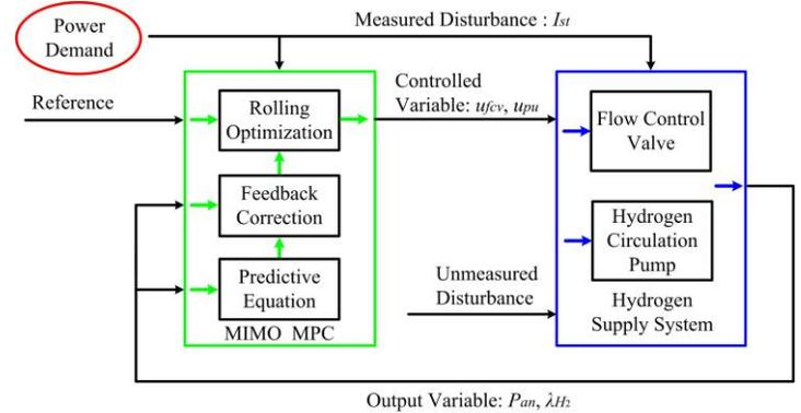
Fig 1 MPC controller structure
