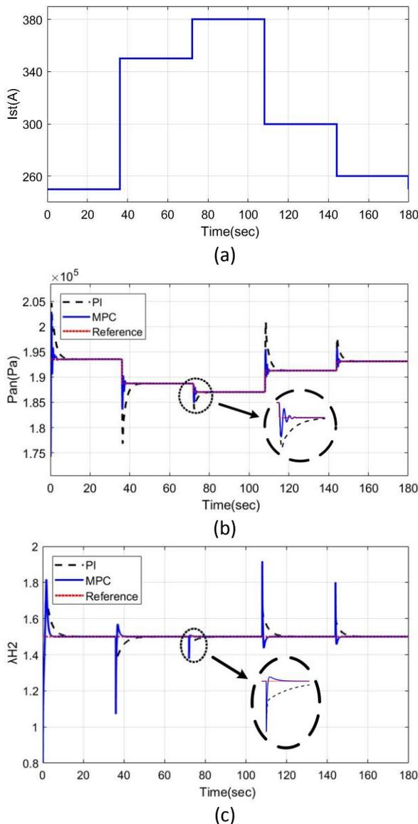
Fig 2 Control results (a) Step change of current (b) pressure of anode (c) hydrogen excess ratio
