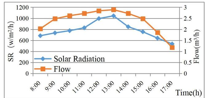
Fig 2 Diurnal variation of solar radiation and water flow in July
