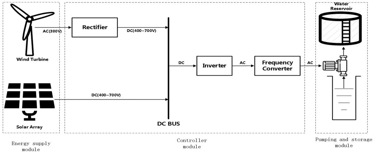
Fig 1 Schematic diagram of wind-solar complementary water supply technology
