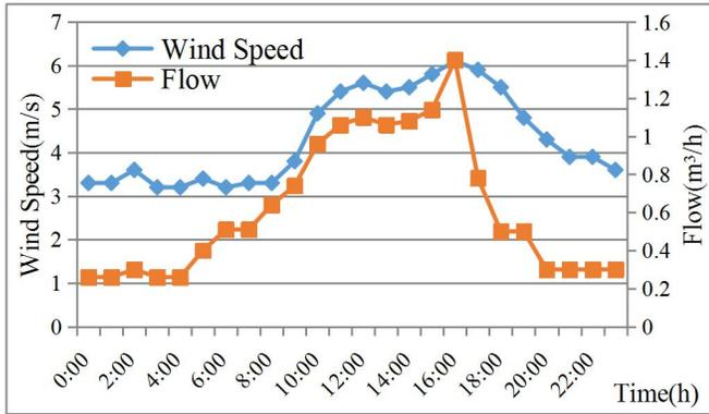
Fig 5 Diurnal variation of wind speed and flow in July
