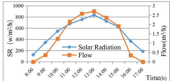
Fig 3 Diurnal variation of solar radiation and water flow in December
