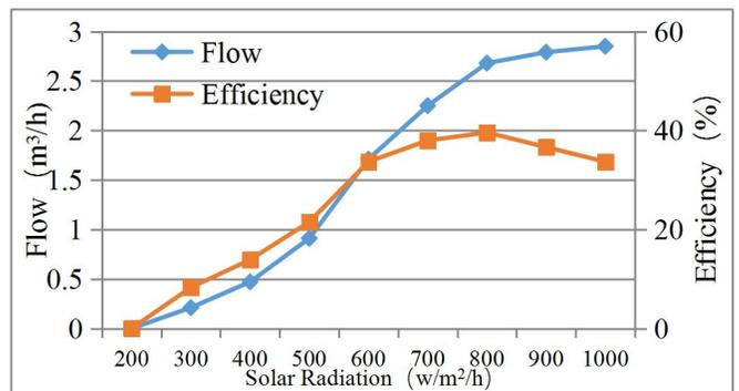
Fig 4 Characteristic of 3 kW solar water pumping system
