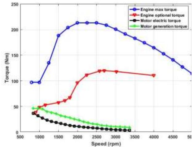
Fig 3. Engine and motor characteristic curves
