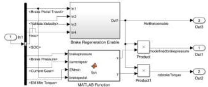
Fig 5. The torque distribution strategy during braking
