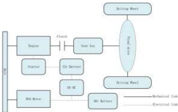
Fig 1. 48V system structure
