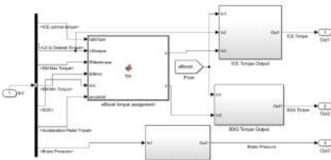
Fig 4. The torque distribution strategy during power assisting
