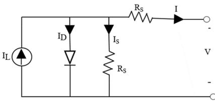
Fig 1 Solar cells model equivalent circuit
