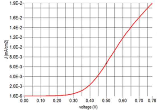
Fig 5 The J-V curve for the optimized Cu<sub>2</sub>O/TiO<sub>2</sub> pn heterojunction
