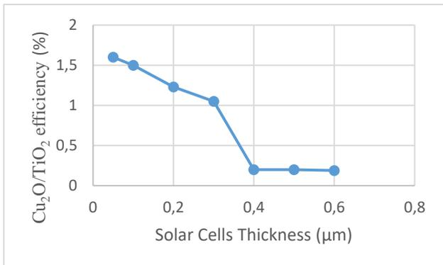
Fig 4 A plot of absorber and buffer layer thickness with the efficiency of the solar cells.
