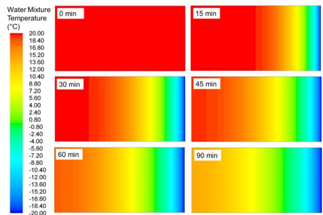
Fig 6 Temperature contours of water mixture in a crystallizer with radial directional freezing at a temperature of -20°C
