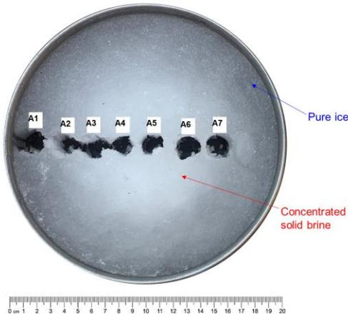
Fig 4 Radially frozen salt-water solution (Sol. A) and samples locations, total volume ~1570mL frozen at -20°C for 24 hours
