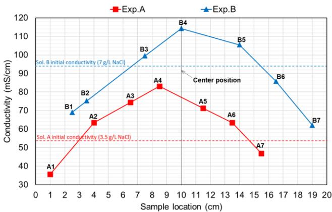
Fig 5 Conductivity results of samples of Sol. A and Sol. B taken at different locations
