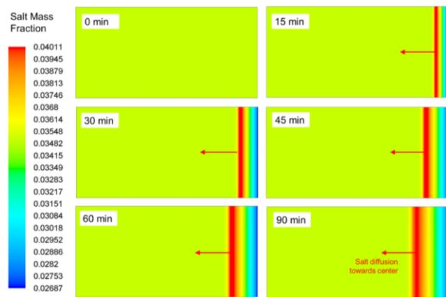
Fig 8 Contours of salt mass fraction showing the salt diffusion towards the center of the crystallizer running at freezing temperature of  $-20^{\circ}\text{C}$
