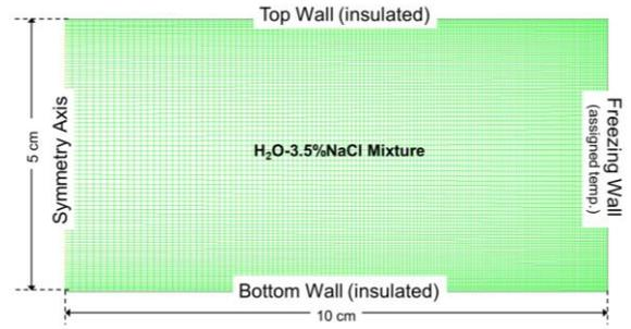
Fig 3 Discretized mesh and assigned boudary conditions
