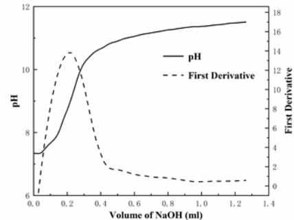
Fig. 2 Curve of Zn-cyclen complex solution titrated by NaOH.
