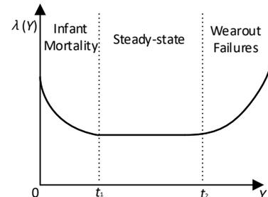
Fig.1 Bathtub curve of pole failure rate.
