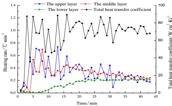
(e) The environment temperature -10°C TS8% inside dish tube heating
