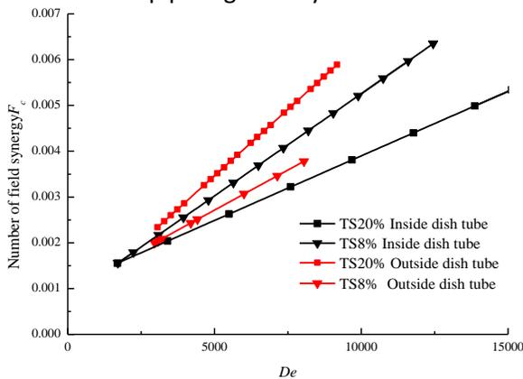
Fig. 5 The field synergy of internal and external coils varies with  $De$  at different TS concentrations
