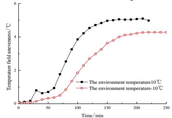
(c) TS20% internal coil heating
