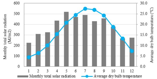
Fig 2 Monthly total solar radiation and average dry bulb temperature in Shanghai.
