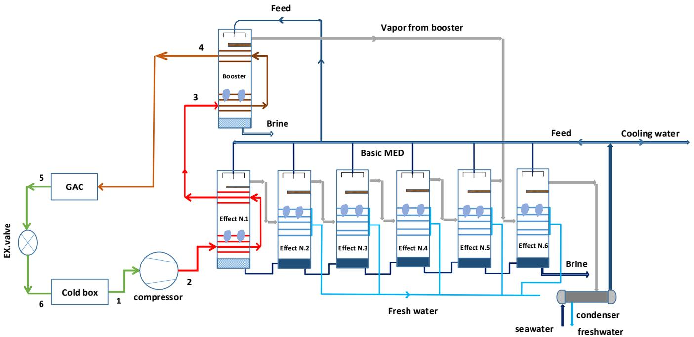
**Fig 1** Schematic diagram of the combined B-MED system with trans-critical carbon dioxide refrigeration system (base system).
