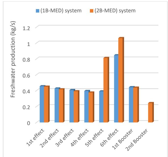
**Fig 4** Comparison of the MED's fresh water production rate of the 2B-MED with that of 1B-MED.
