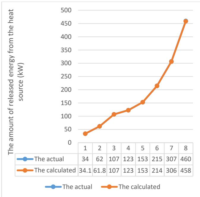
**Fig 3** Comparison of the calculated amount of released energy from the heat source and the actual amount of released energy from Alfa Laval single effect freshwater generators.
