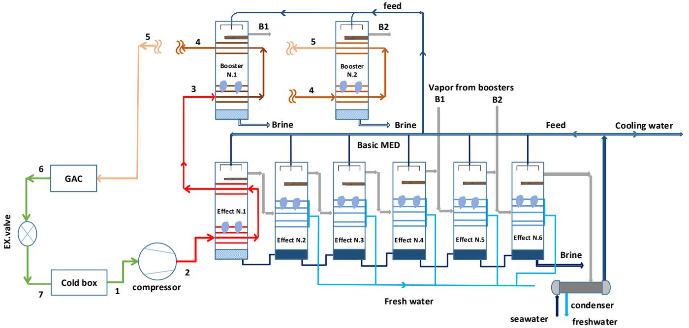
Fig 2 Schematic diagram of the combined system with two Booster Modules (the optimized system).
