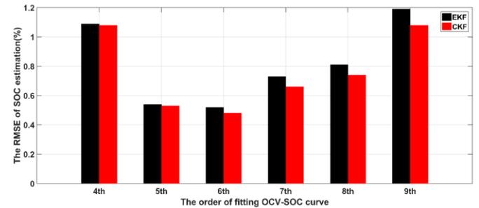
Fig 7 Relationship between the order of fitted OCV-SOC curve and SOC-RMSE.
