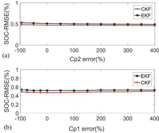
Fig 5 Influence of polarization capacitors on SOC estimation: (a)  $C_{p2}$ ; (b)  $C_{p1}$ .
