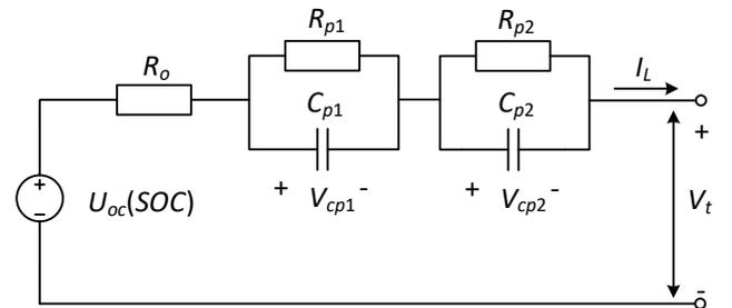
Fig 2 Schematic of second-order RC model.
