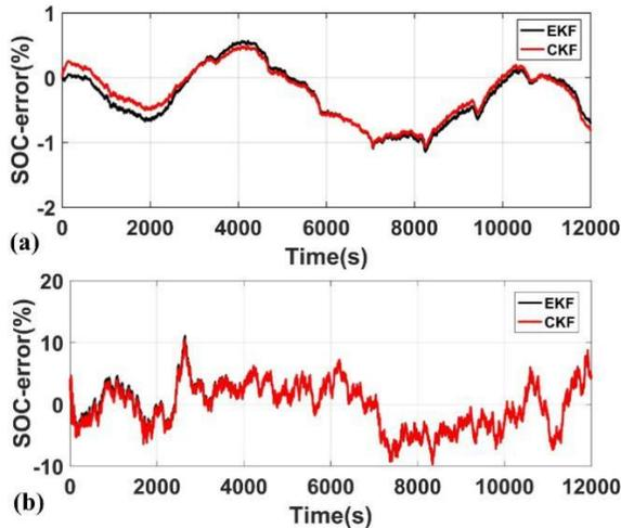
Fig 8 RMSE of SOC estimation with measurement noises: (a) current noise; (b) voltage noise.
