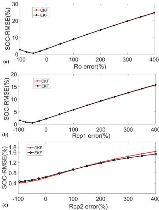
Fig 6 Influence of resistors on SOC estimation: (a) Ohmic resistor  $R_o$ ; (b) polarization resistor  $R_{p1}$ ; (c) polarization resistor  $R_{p2}$ .
