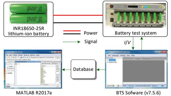
Fig 1 Configuration of the battery test bench.
