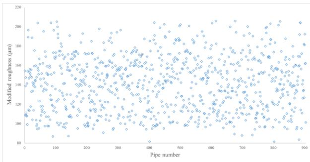
Fig.3 The calibrated value  $\epsilon_m$  of all pipes
