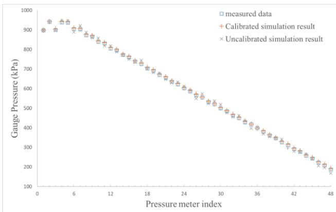
Fig.5 The estimated pressure results and measured data
