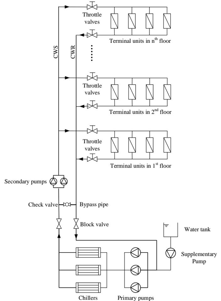
Fig.1 The configuration of a chilled water system
