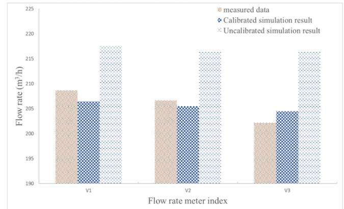
Fig.6 The estimated flow rate results and measured data
