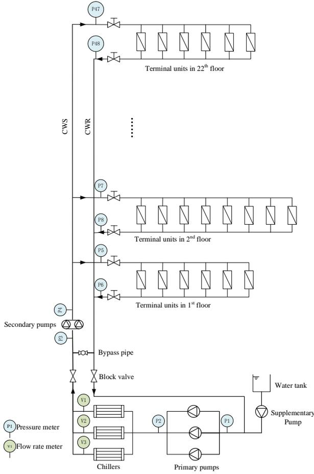
Fig.2 The configuration of a chilled water system in a high-rise building of 22 floors
