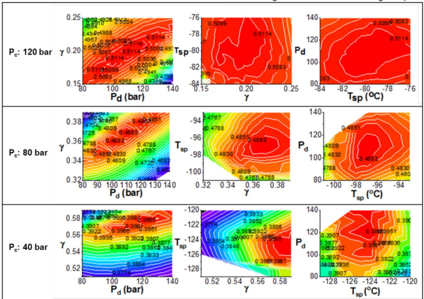
Fig 2 Overall efficiency versus  $P_d$ ,  $\gamma$ , and  $T_{sp}$  panel contour graphs at  $P_c = 40, 80,$  and  $120$  bar
