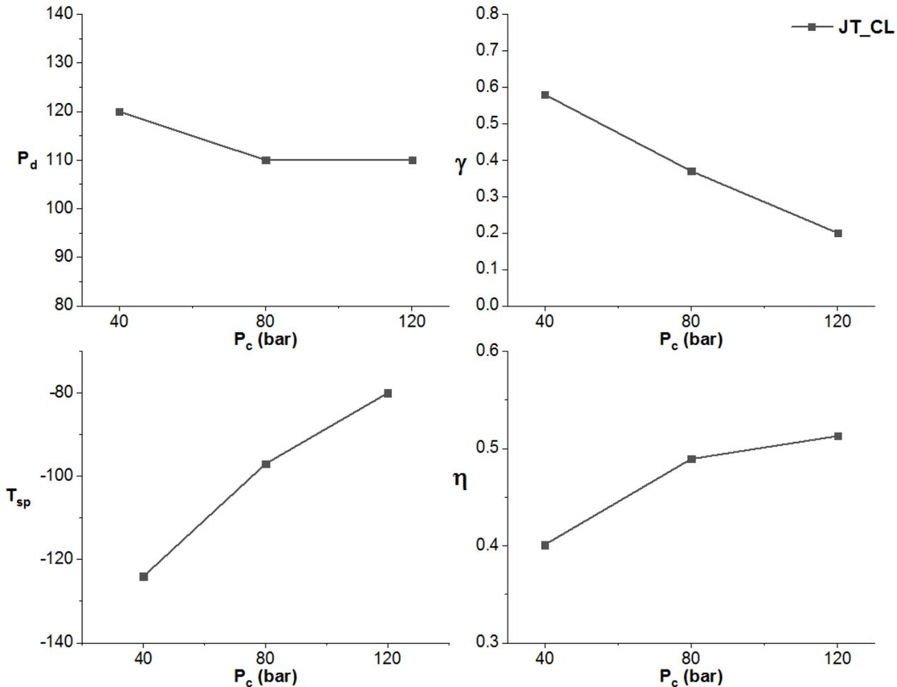
Fig 3 Optimal values of  $P_d$ ,  $\gamma$ , and  $T_{sp}$ , and overall efficiency at different  $P_c$
