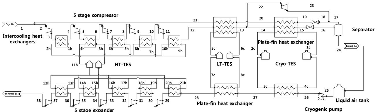
Fig 1 Process flow diagram of LAES with modified Kapitza cycle
