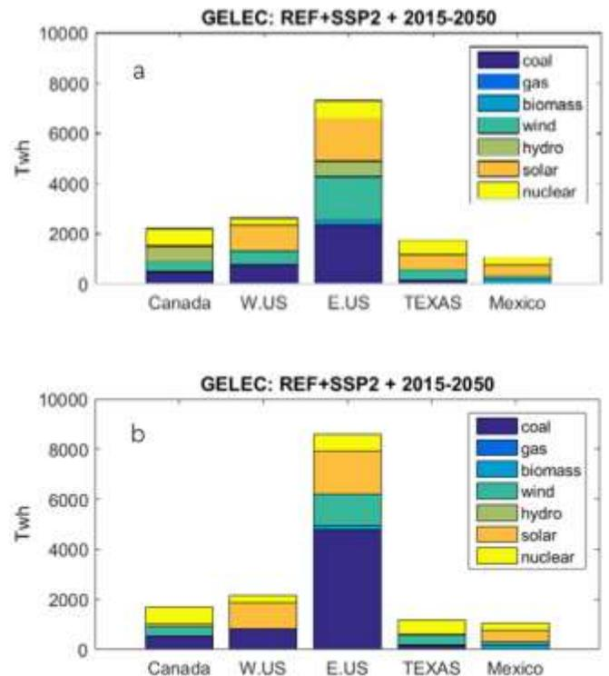
Fig 3 The electricity supply structure of Canada-USA-Mexico under 2 interconnection scenarios. (a, Weak Connection; b, Strong Connection)
