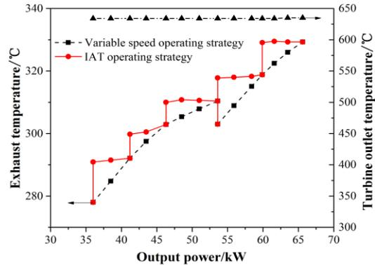
Fig 4. Turbine outlet temperature/exhaust gas temperature with different operating strategies
