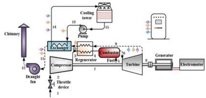
Fig 1. Schematic configuration of the experimental rig.
