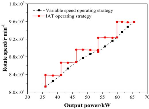
Fig 3. Rotate speed of the gas turbine with different operating strategies
