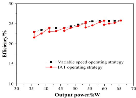
Fig 6. Efficiency of the gas turbine with different operating strategies
