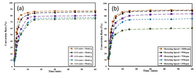
Fig 2 The carbonation conversion under various (a) LSR (b) rotating speed.
