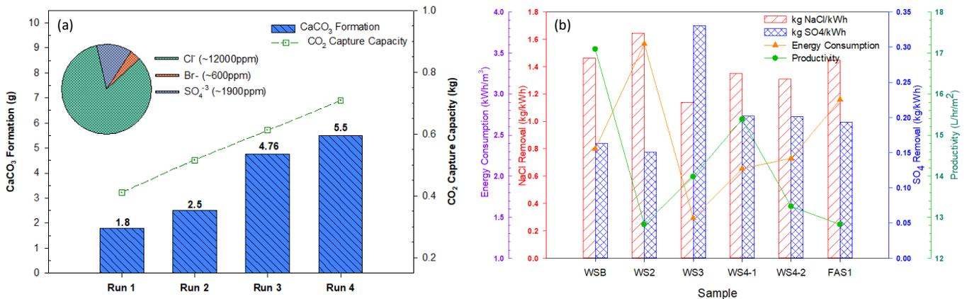
Fig 3 (a) Performance of  $\text{CaCO}_3$  formation,  $\text{CO}_2$  capture capacity and anions of leachate during indirect carbonation; (b) Performance of energy consumption, anion removal and productivity for FA leachate treatment via RW-EDI.
