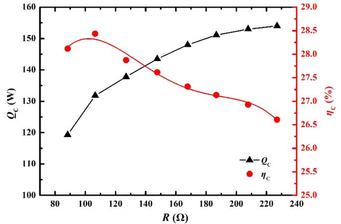
Fig. 4 Cooling power and relative Carnot efficiency vs. load resistance
