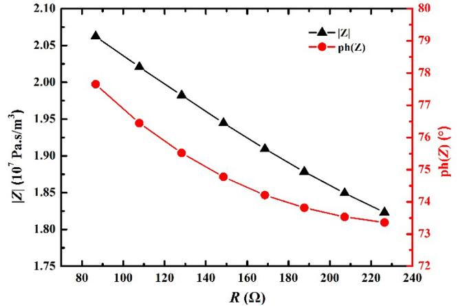
Fig. 3 Acoustic impedance magnitude and argument of linear motor vs. load resistance
