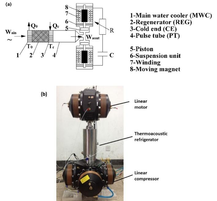
Fig. 1 Experimental apparatus: (a) schematic, (b) photograph
