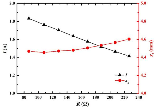
Fig. 5 Current and piston displacement of linear motor vs. load resistance
