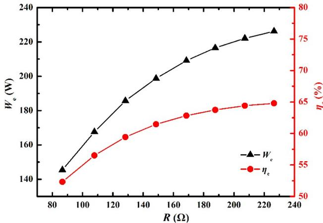
Fig. 6 Electric power and efficiency of linear motor vs. load resistance
