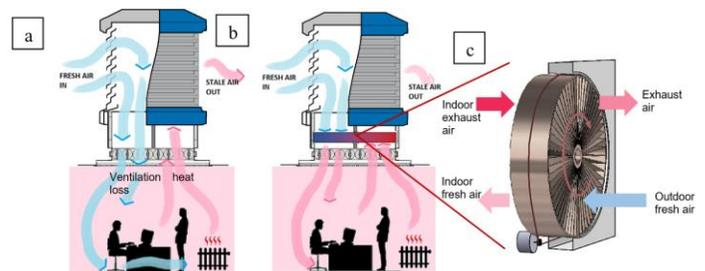
Fig 1 (a) standard windcatcher (b) passive heat recovery windcatcher (c) proposed passive heat recovery wheel
