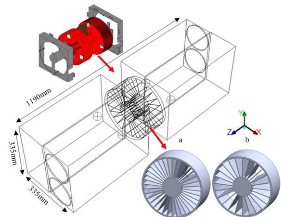
Fig 2 Computational model of the two-way cross-flow duct used for evaluating the performance of (a) 32- and (b) 20-radial blade arrangement
