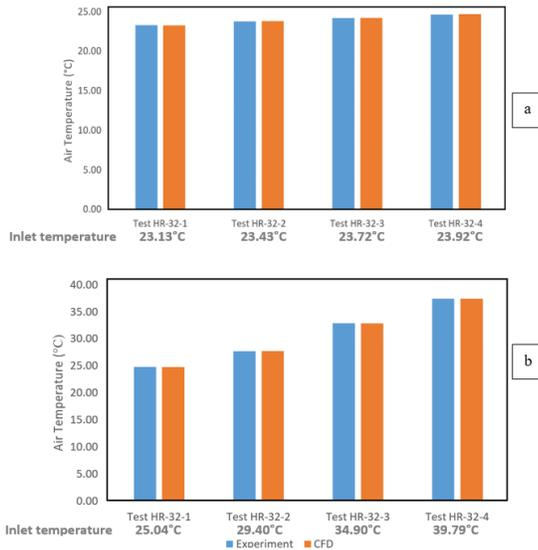
Fig 6 Comparison between experiment and CFD air temperature in the (a) incoming and (b) outgoing airstream after the 32 blade rotary wheel.
