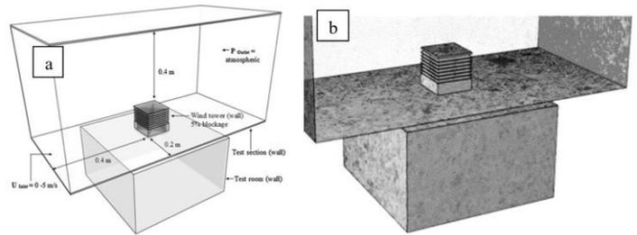
Fig 4 (a) Computational domain (b) mesh around the surfaces of the model arrangement
