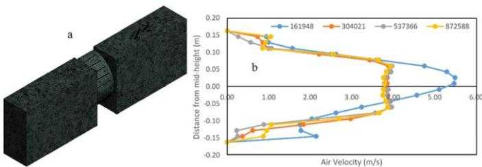
Fig 3 (a) Computational mesh (b) mesh sensitivity analysis
