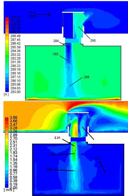
Fig 7 Cross-sectional contour planes of (a) air temperature (b) air velocity with the outdoor wind speed and temperature at 3m/s and 283K
