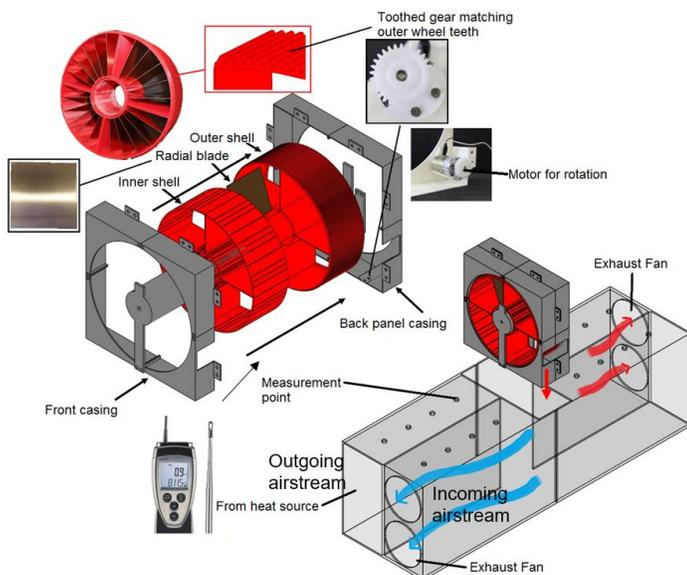
Fig 5 Experimental setup of the passive heat recovery wheel test
