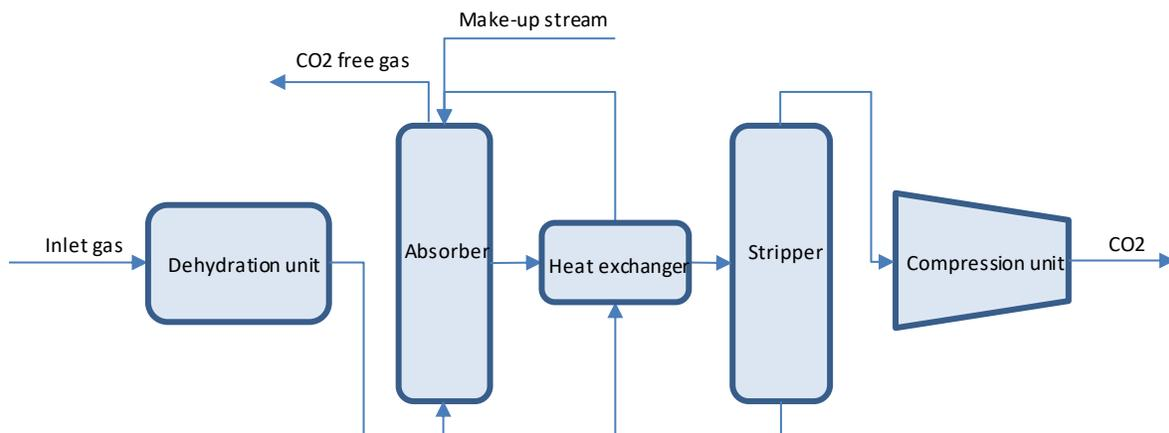
Fig 1 Schematic diagram of MEA-based CO<sub>2</sub> capture process
