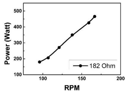
Fig 8 The power output of a PMSG installed in the FKT in the towing tank
