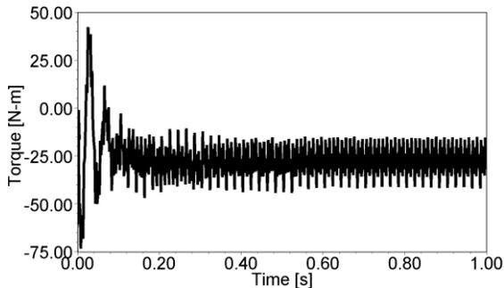
Fig 2 Simulated torque of the PMSG at 150 rpm with a load of 182 Ohm
