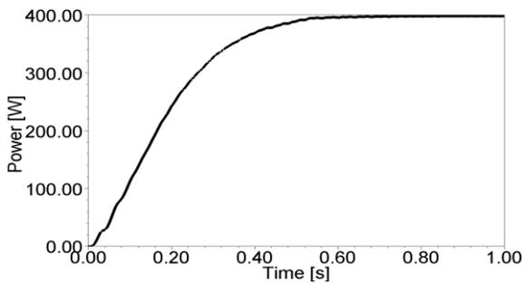
Fig 1 Simulated DC power after rectifier
