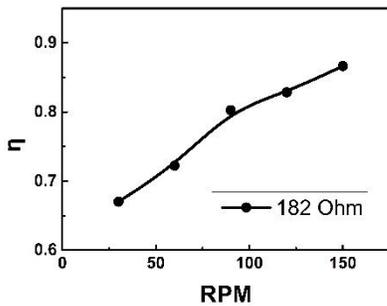
Fig 6 Energy conversion efficiency of the tested PMSG in the testing platform
