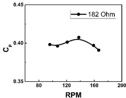
Fig 9 The power coefficient (Cp) of FKT system from towing tank
