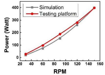
Fig 3 Simulated and tested DC power output of the PMSG at different rpm
