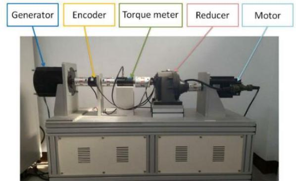
Fig 4 Illustration of the testing platform [16]
