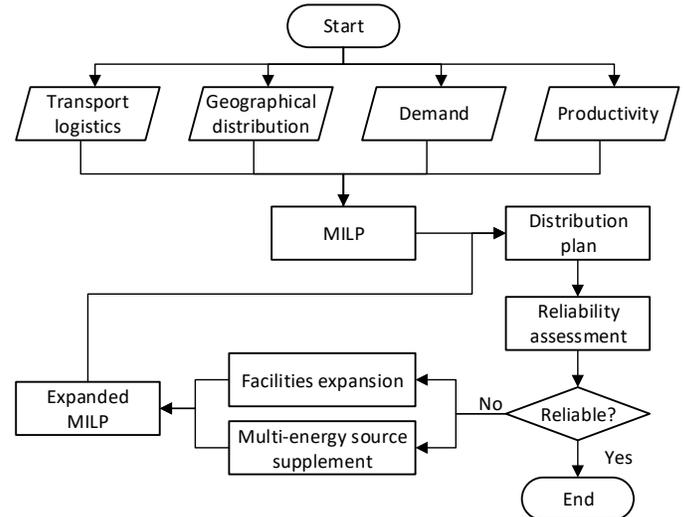
Fig 2 Flowchart of the designed framework for flexible RPSC research
