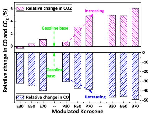
Figure 6 Relative change in CO and CO<sub>2</sub> compared with base gasoline for nine modulated kerosene
