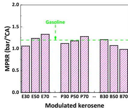
Figure 4 Comparison of the MPRR between gasoline and modulated kerosene
