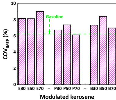
Figure 5 The CoV<sub>IMEP</sub> of gasoline and modulated kerosene
