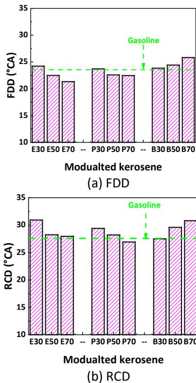
Figure 3 Comparison of FDD and RCD between gasoline and modulated kerosene
