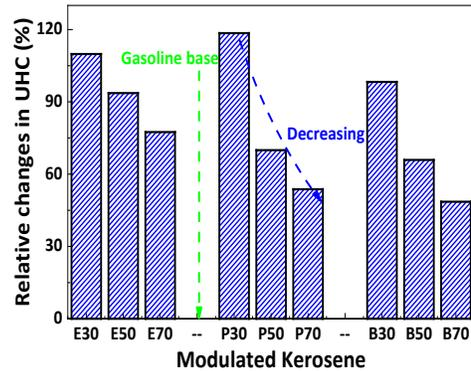
Figure 7 Relative change in UHC emissions compared with base gasoline for nine modulated kerosene
