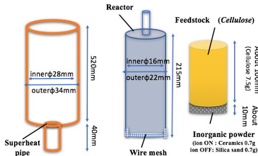
Fig 3. The structure of the heating pipe and inner pipe
