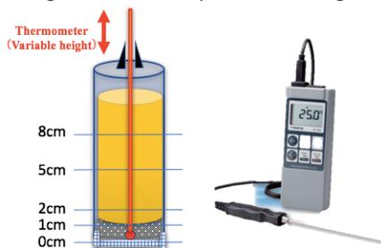
Fig.5 Temperature measurement positions and equipment
