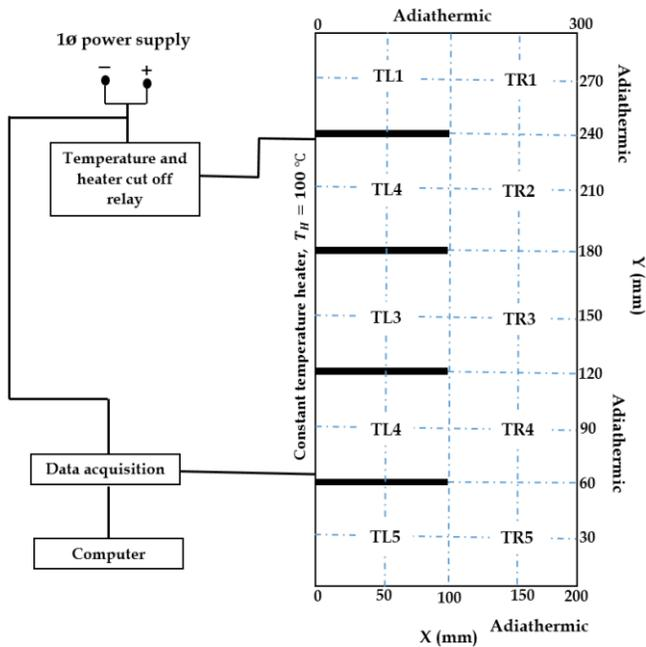
Figure 1: Experimental setup schematic for a LHTES system associated with fins
