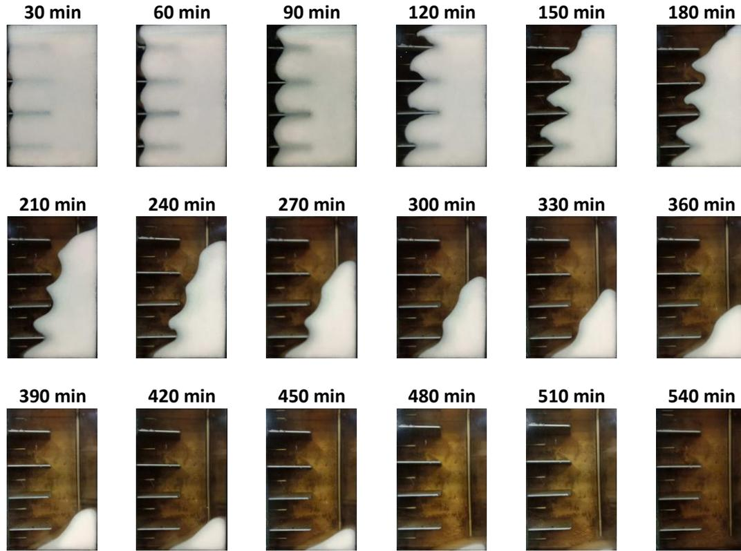
Figure 2: Temporal evolution of liquid-solid interface during melting process
