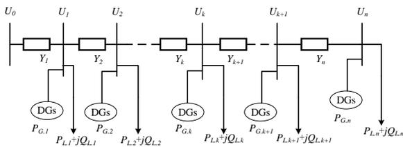
Fig.1 Power system model with distributed PV
