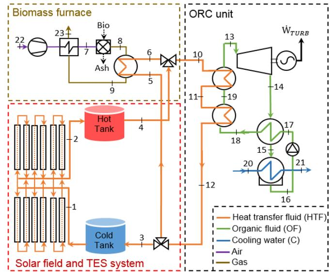
Fig 1 Conceptual scheme of the hybrid CSP-biomass ORC plant
