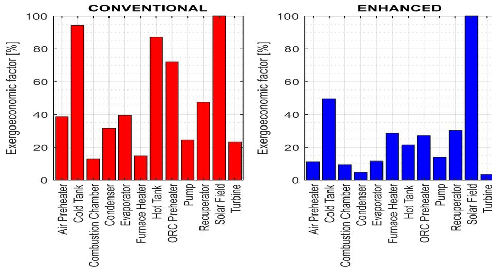
Fig 2 Comparison of conventional and enhanced exergoeconomic factors for the hybrid solar-biomass plant
