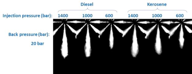
Fig.6 Spray evolutions for diesel and kerosene
