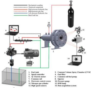
Fig.1 Experimental setup for spray study
