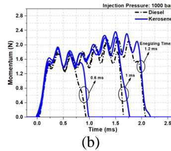
Fig.4 Comparison of spray momentum for diesel and kerosene
