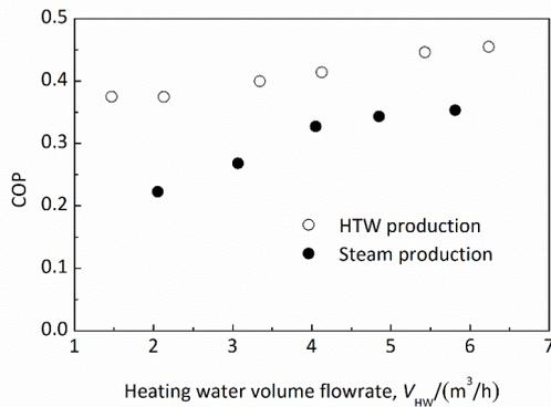
Fig 7 COP versus heating water volume flowrate for production of HTW and steam
