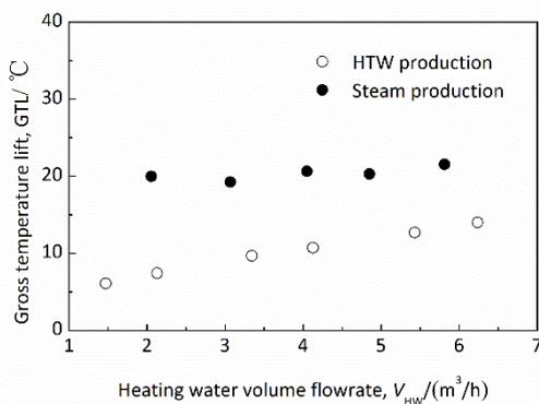
Fig 8 Gross temperature lift versus heating water volume flowrate for production of HTW and steam
