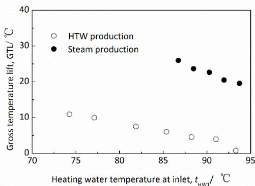
Fig 5 Gross temperature lift versus heating water temperature for production of HTW and steam
