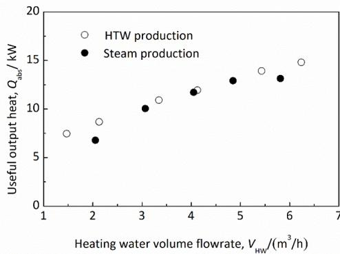
Fig 6 Useful output heat versus heating water volume flowrate for production of HTW and steam
