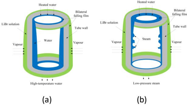
Fig 2 Distribution of liquid film of bilateral falling film absorber (a) HTW production (b) steam production
