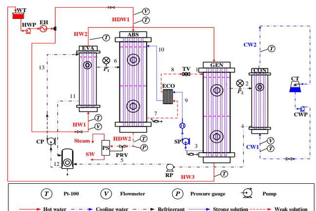
Fig 1 Diagram of the experimental SSHT in this study
