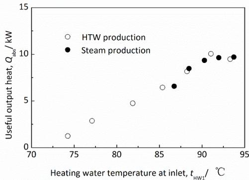
Fig 3 Useful output heat versus heating water temperature for production of HTW and steam
