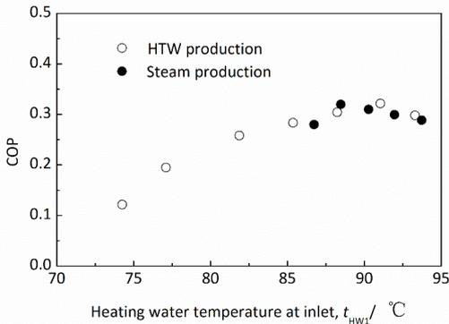
Fig 4 COP versus heating water temperature for production of HTW and steam
