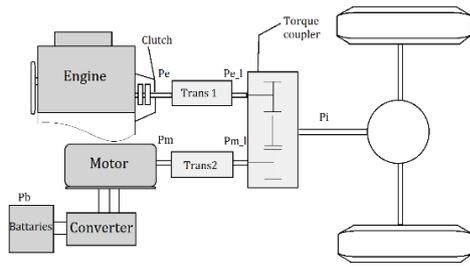
Fig. 5 Configuration of a full-size-engine parallel HEV [19]
