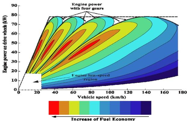
Fig. 7 Fuel consumption map for a typical 80 kW ICE in various gear ratio to the drive wheel [19]
