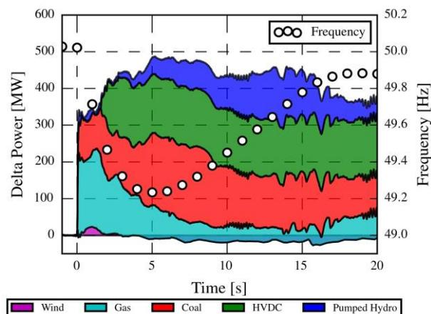
Fig. 1 Observed and extrapolated generation to a 420 MW loss of generation on the Irish power system
