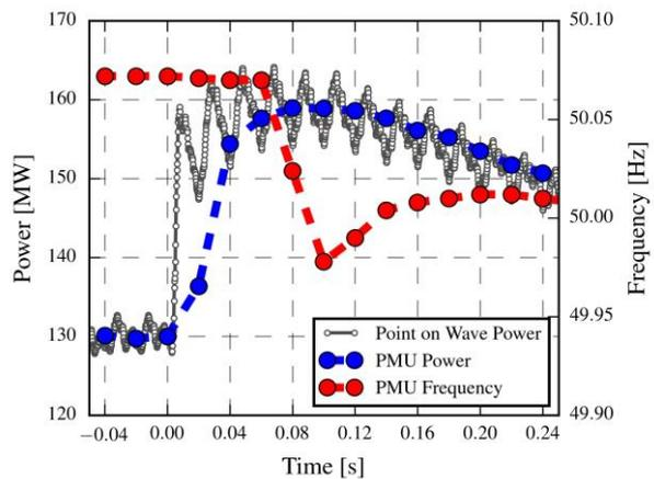
Fig 3, Capture of the initial response of a CCGT synchronous generator to a significant frequency transient.
