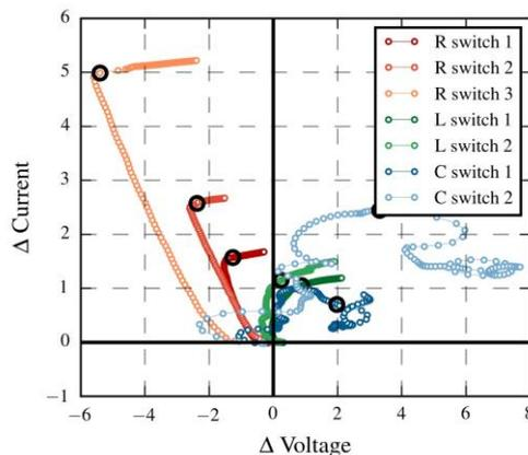
Fig 4, Change in voltage and current output from a laboratory synchronous generator during the first 20 ms post transient events [12] (the black circle marks 10 ms post event)
