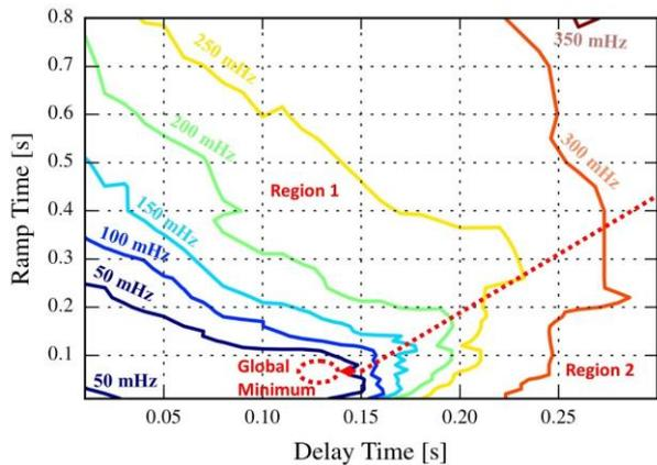
Fig 2, Effect of delay time and ramp time on RoCoF
