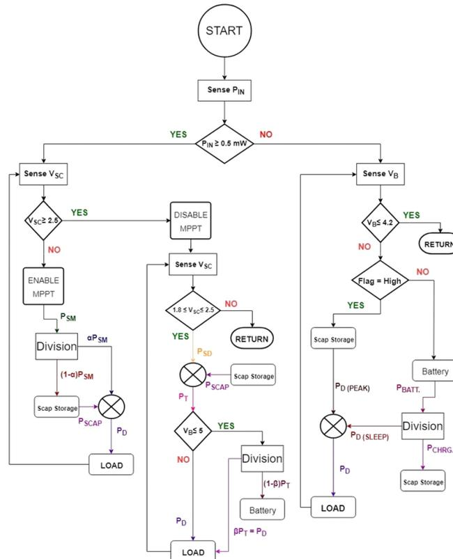
Figure 2 Power Management Algorithm (PMA)
