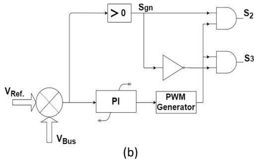
Figure 1 (a) Proposed power management circuit diagram (b) controller design for supercapacitor converter
