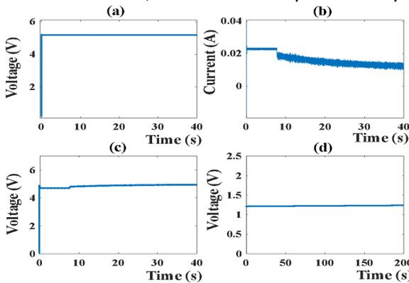
Figure 3 Simulation results for the system operating in Day Mode-1, (a) PV voltage, (b) PV current, (c) Load Voltage, (d) Supercapacitor voltage
