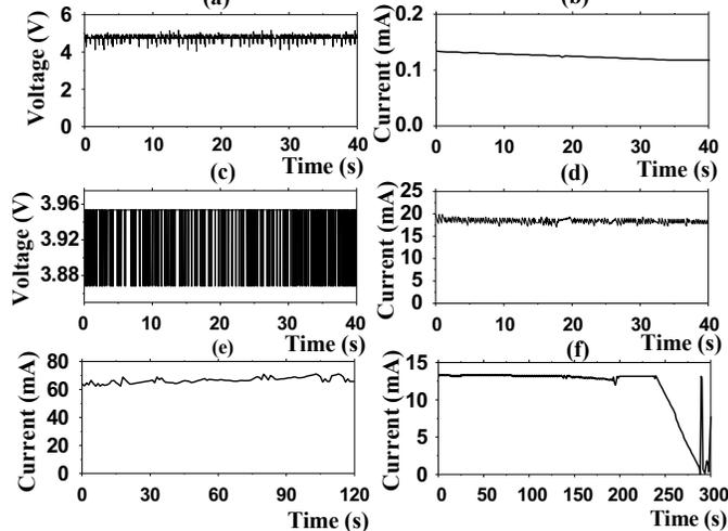
Figure 6 Experimental results for the system operating under the Day Mode-2, (a) PV and Load voltage, (b) PV current, (c) Battery voltage, (d) Battery charging current, (e) Peak Load current, (f) Battery discharge current
