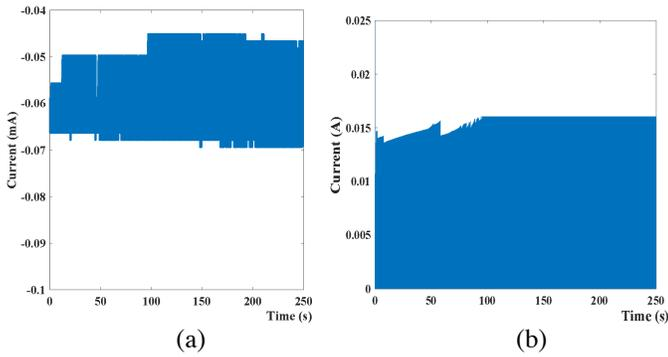
Figure 5 Simulation results for the Dark Mode-3,4, (a) Peak load current (b) Battery discharge current
