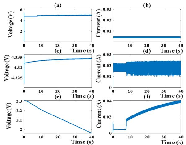
Figure 4 Simulation results for the system operating in Day Mode-2, (a) PV voltage, (b) PV current, (c) Battery voltage, (d) Battery charging current, (e) Supercapacitor voltage and (f) Supercapacitor discharging current
